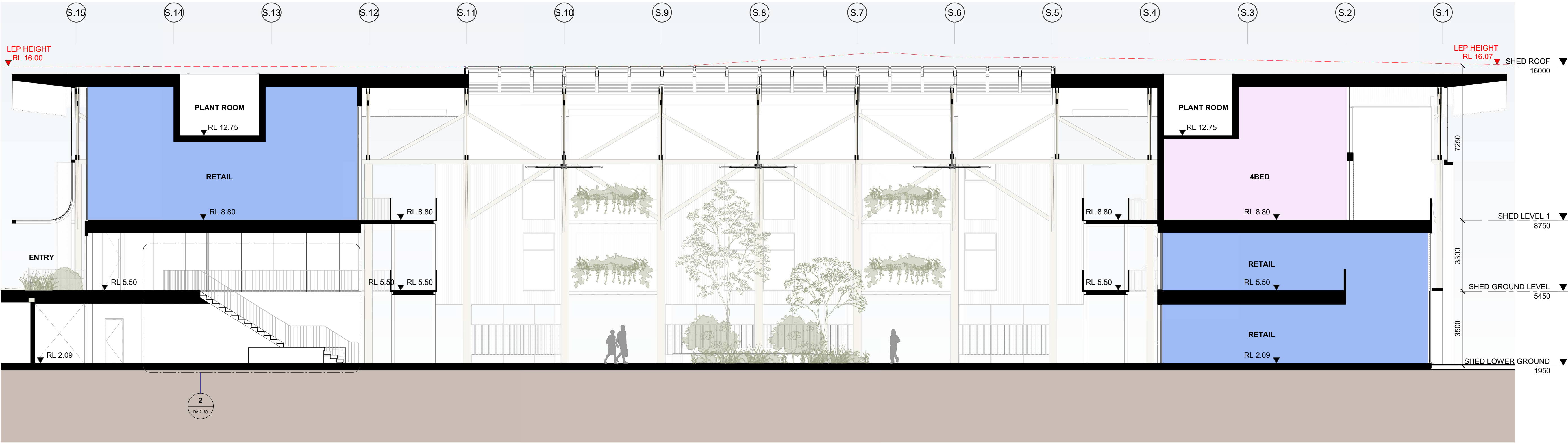
1 N-S SECTION THROUGH SHED SCALE 1:100
